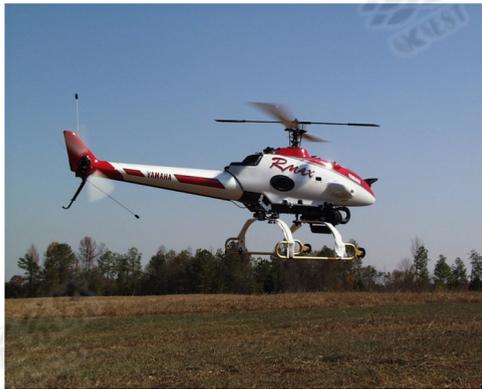
**Fig. 5.** Yamaha R-Max unmanned helicopter used for agricultural spraying (Gtuav, 2014).
