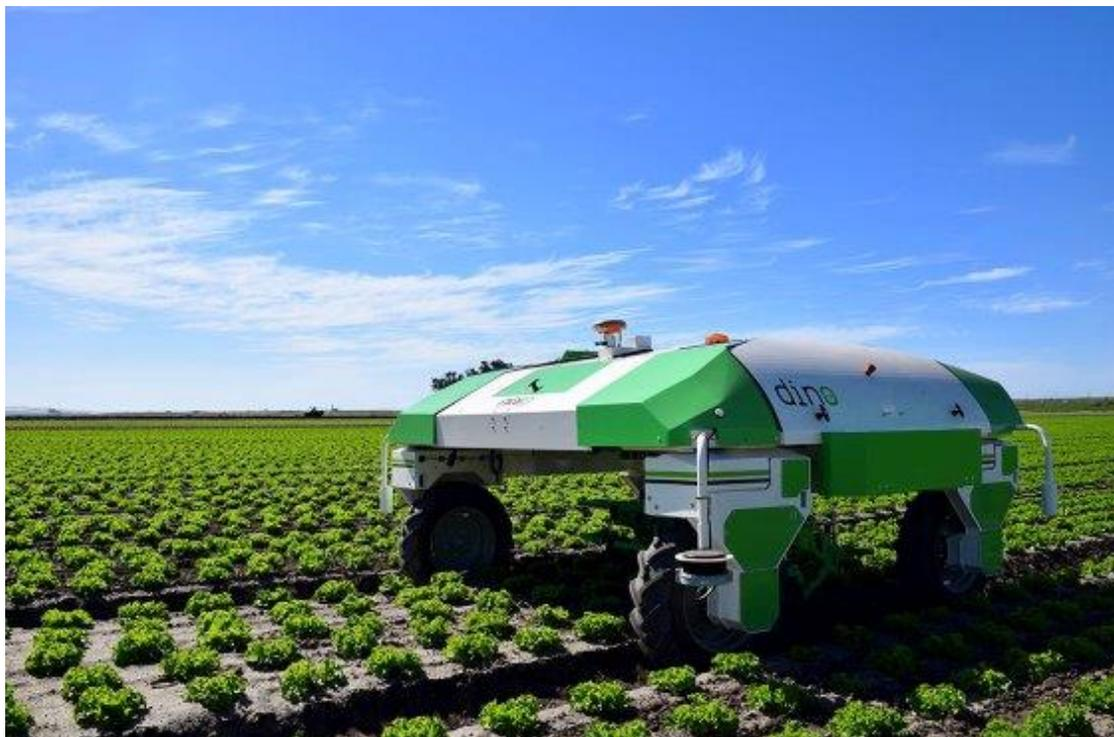
Dino is the first entirely autonomous electric robot to mechanically weed vegetable crops. The robot is designed by Naïo Technologies and has been on the market since early 2017. - Photos: Naïo Technologies
