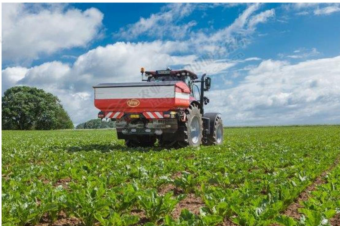
Top-spec Vicon Rotaflow twin-disc spreaders with Geospread capability can now offer a more refined variable rate technology that gets closer to target rates at precision map boundaries by adjusting rates within the spread pattern. - Photo: Kverneland
