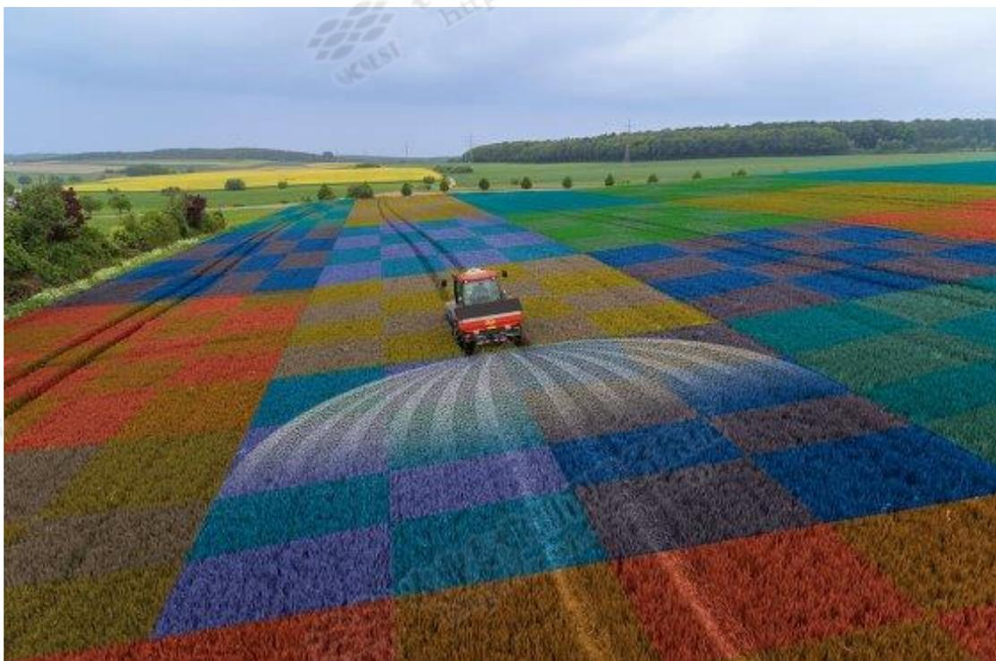
...but with Geospread Multirate, the spread pattern is adjusted within the working width to accommodate up to eight different rates. - Photos: Kverneland
